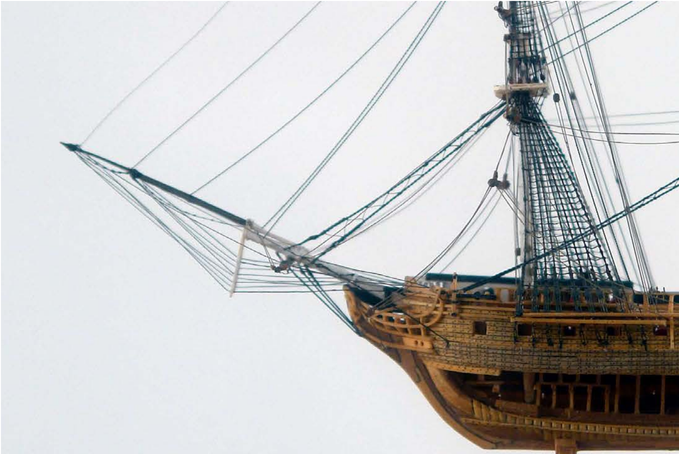
This remarkable model of the USS Constitution is shown here five times its actual size. The frames are made of magnolia, with double 'bends' to represent the full-size framing practice. The keel, stem and sternpost are of apple wood, with three scarph joints in the keel as per the original specifications. The stem is joined to the keel with a compound scarph and is made of five pieces. The interior is fitted with all beams for each deck. The knees, carlings and ledges are fitted to the starboard side only, to allow the fullest view down into the structure from above.
