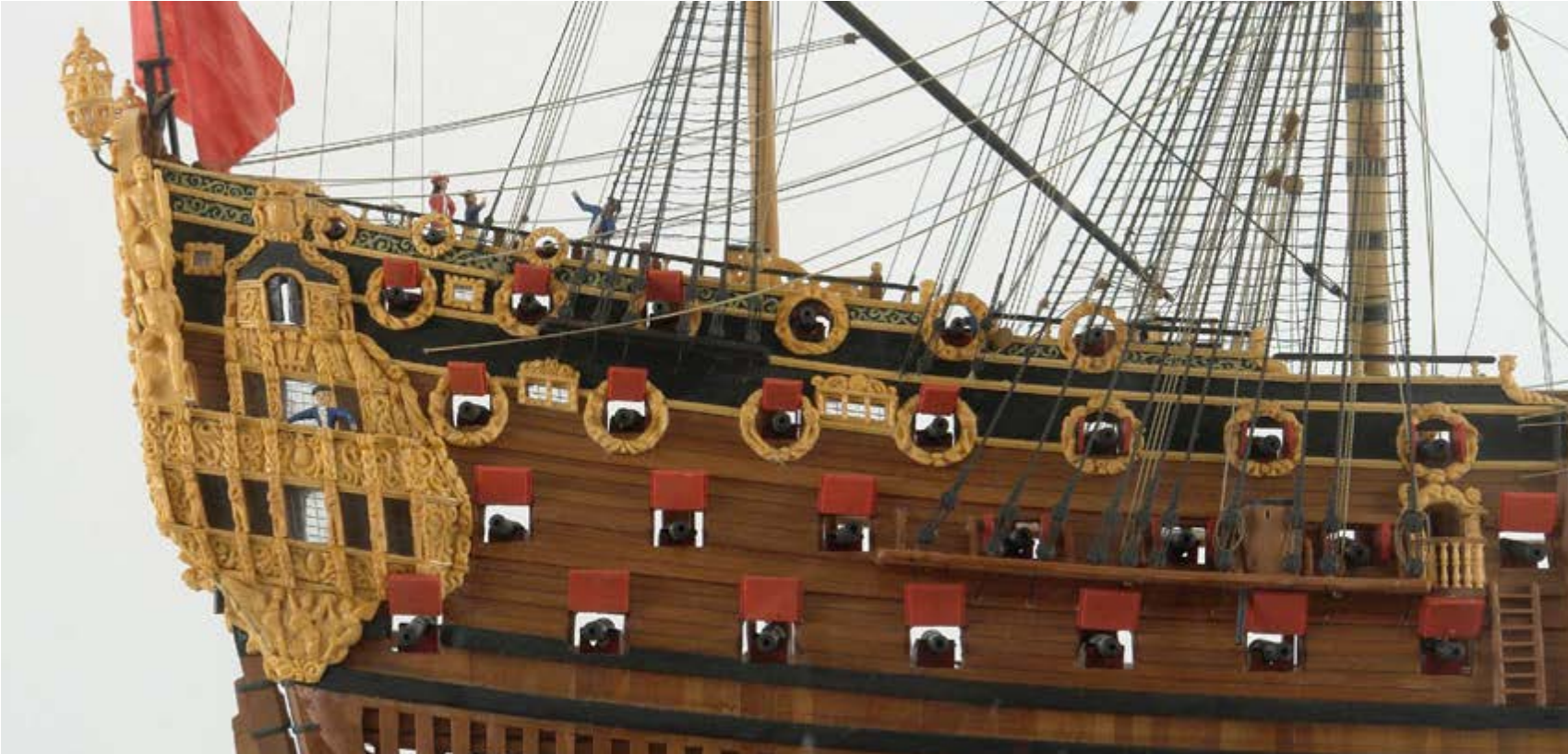
Detail of the starboard side. The guns are painted wood to imitate the original iron. The stanchions of the balustrade on the entry port are just 3/16" high. Those under the cap rail are 3/32" yet all were hand-turned by the artist.
