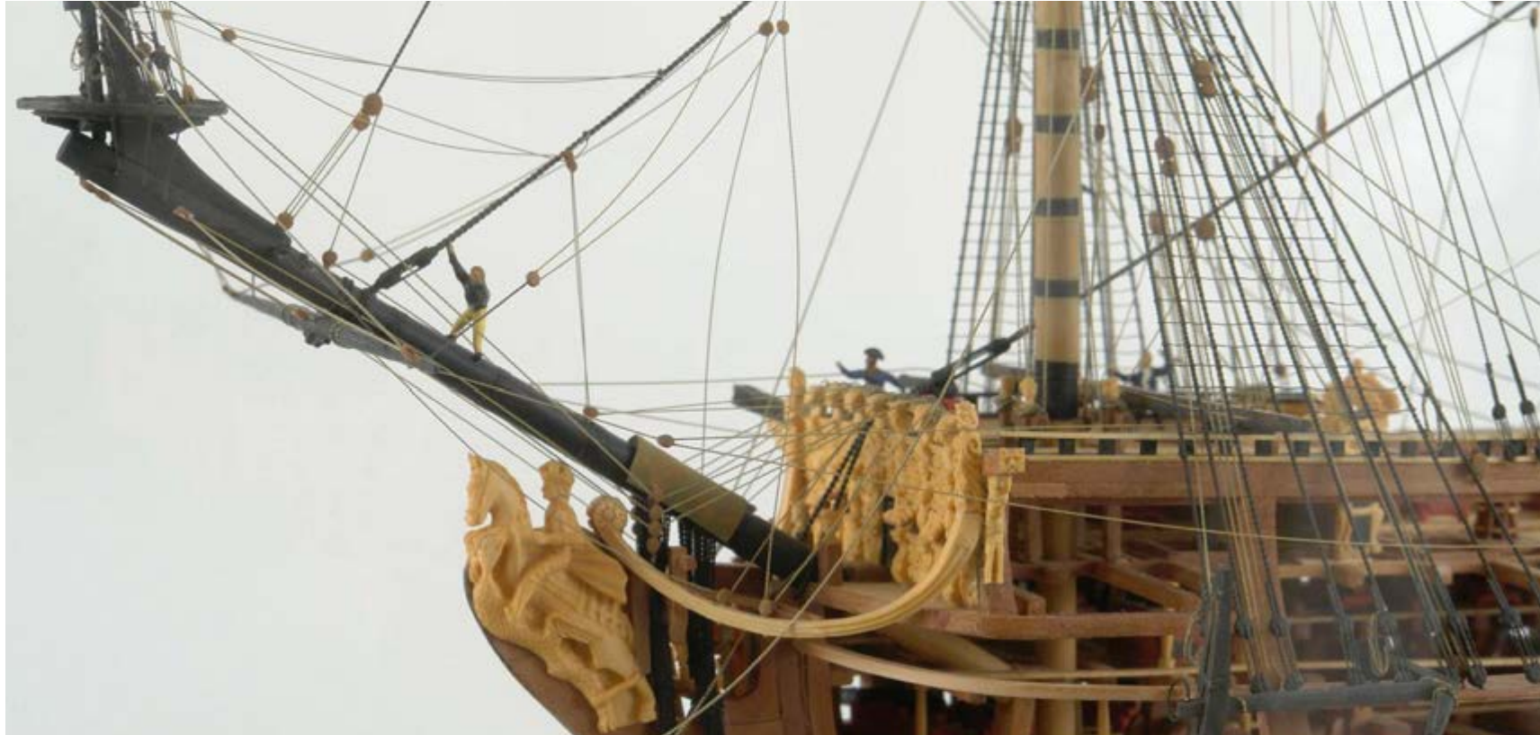
This bow section clearly shows the intricate standing rigging that McCaffery has replicated along with the carved figurehead of King Charles II trampling a dragon and the headrails leading to the elaborate carved beakhead bulkhead showing warrior figures. For scale, McCaffery has included two sailors that give us a sense of how massive the original carvings he's replicated really were.
