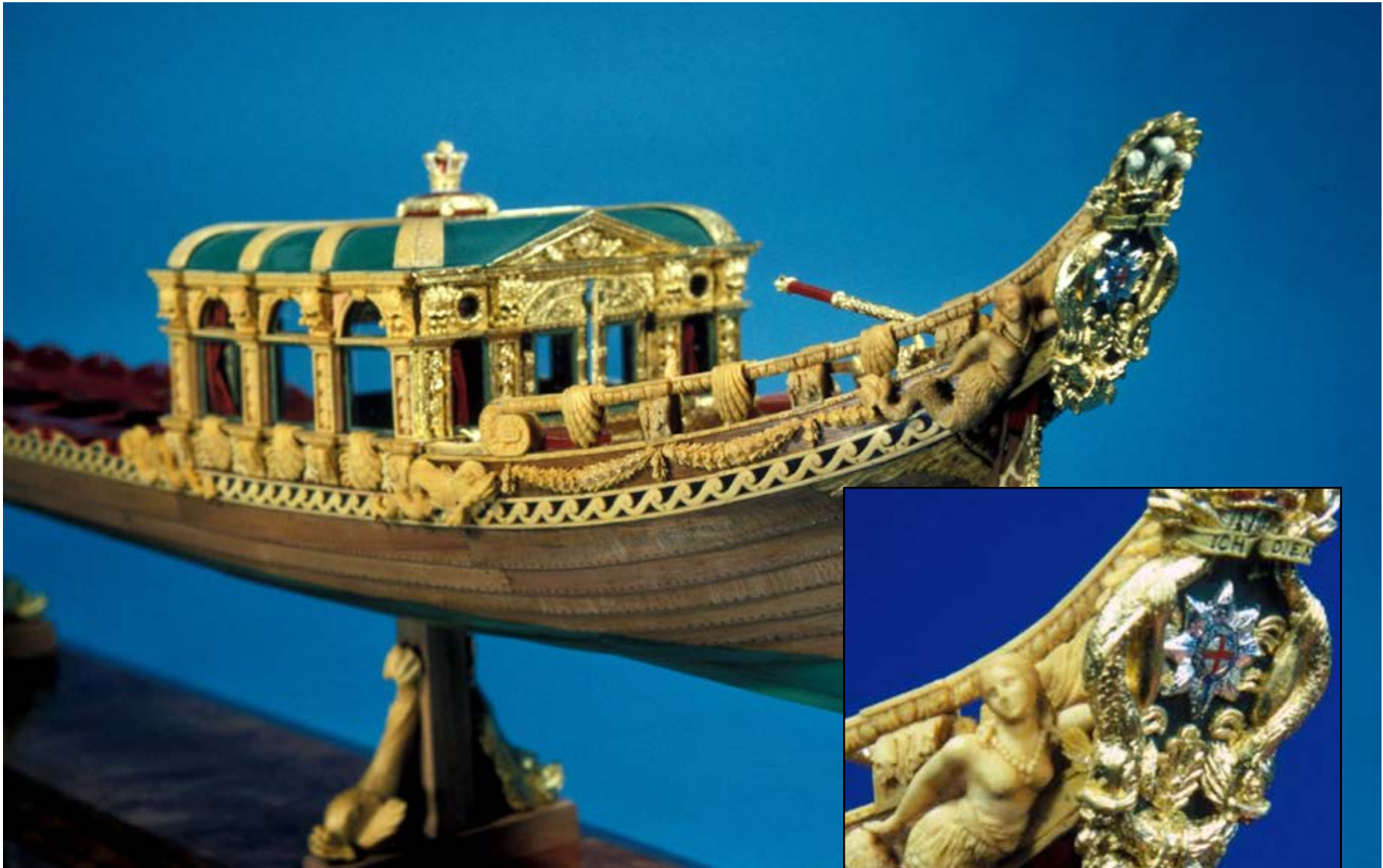
The model's intricate stern features the Garter Star stern emblem shown below the Prince of Wales' feathers. It is constructed of 34 different pieces fitted together then gold-leafed and attached to the hull.
