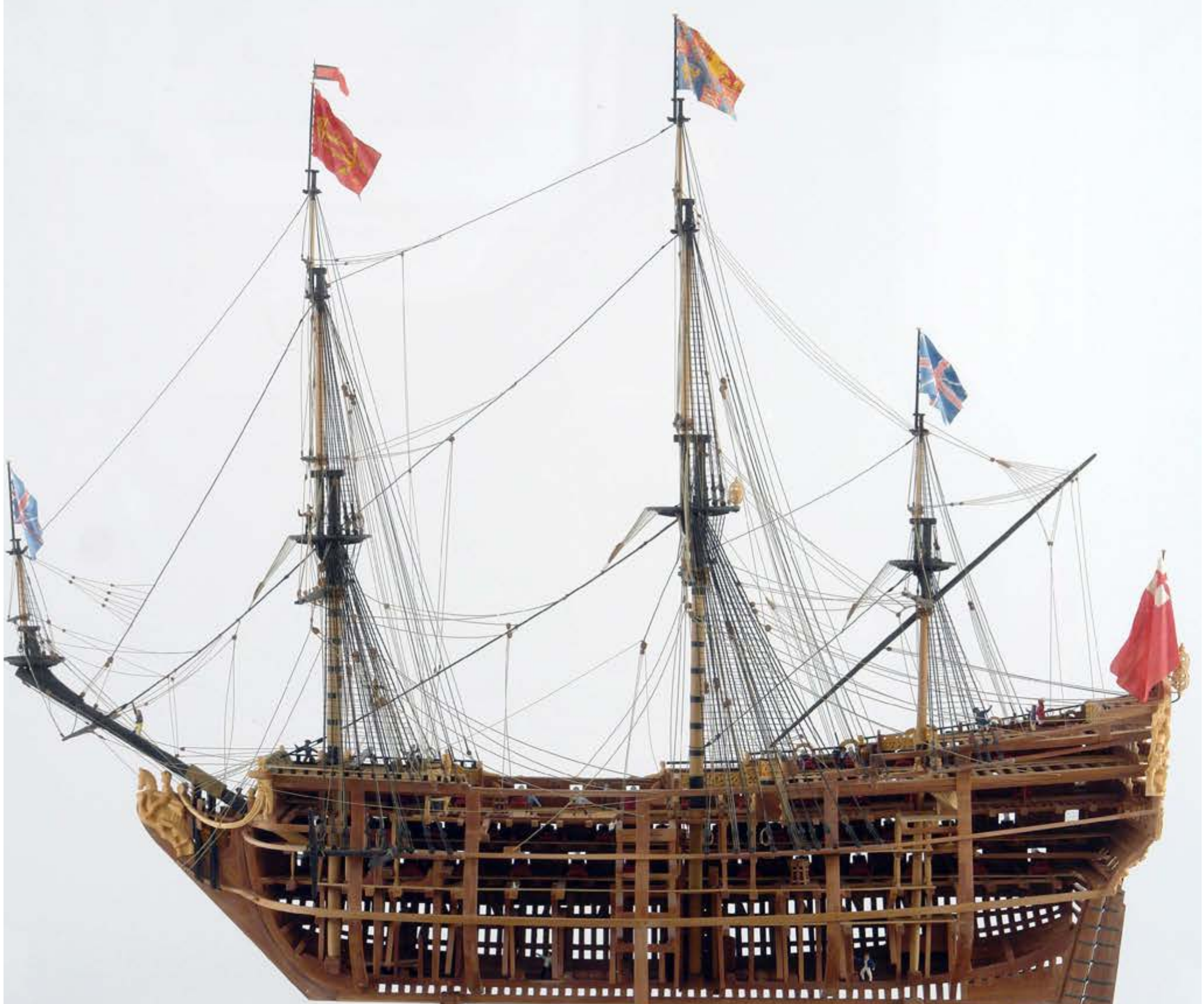
Overview of the port side showing how just five main "bends" serve to define the ship's shape and are held in place by the lower main wale and upper chain wale. The channels, very conveniently, anchor to the wale.
