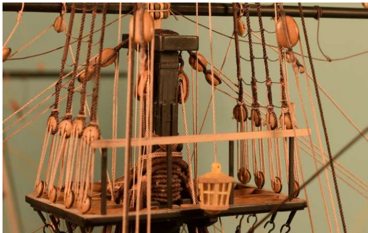
The mast tops are where the intricate standing and running rigging intersect.
