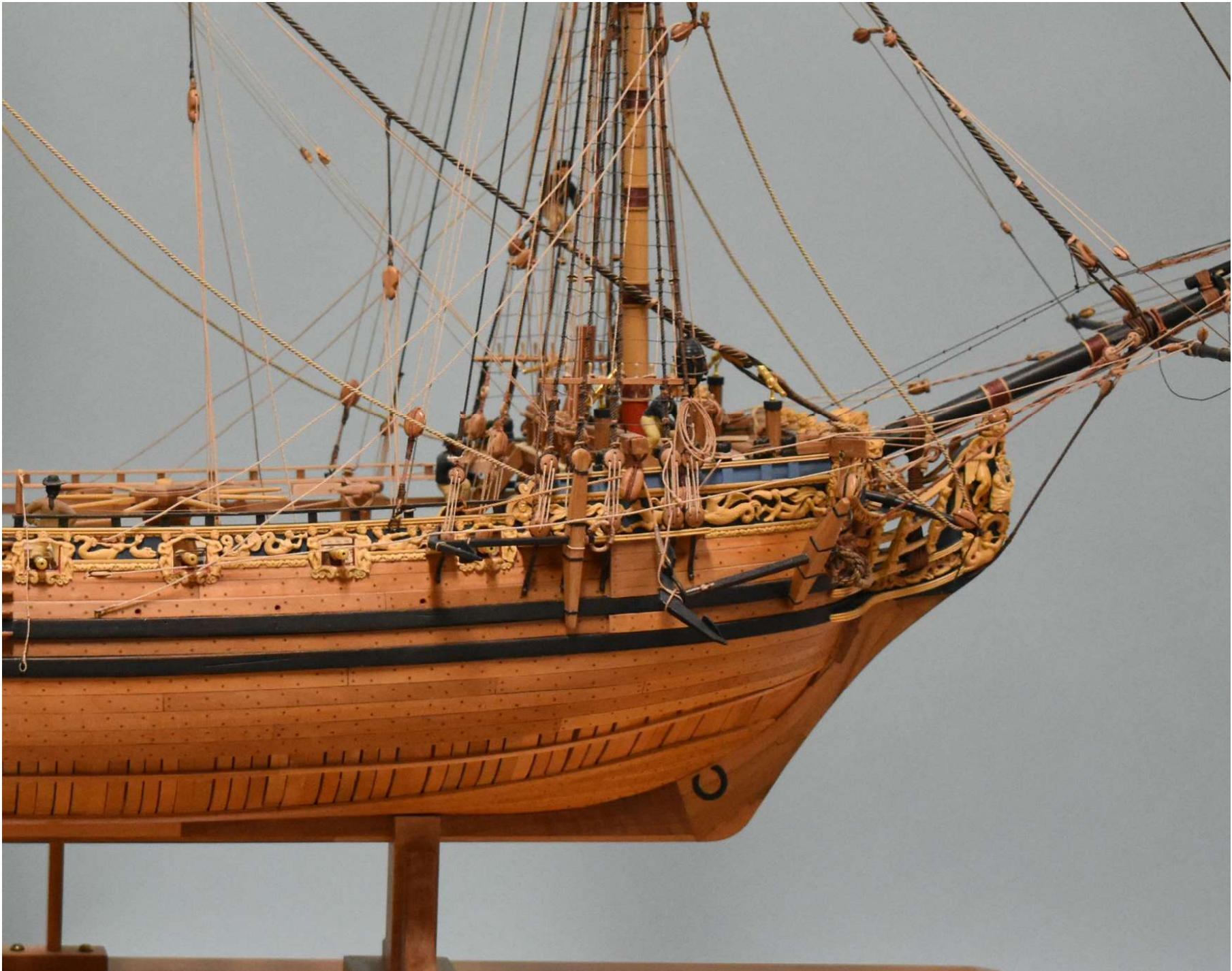
This view of the model shows framing, planking and decorative carvings.
