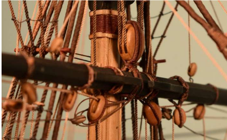
Under the fore top are the "jeers," a massive, complex single and double block assemblage used to lower and hoist the lower yard.
