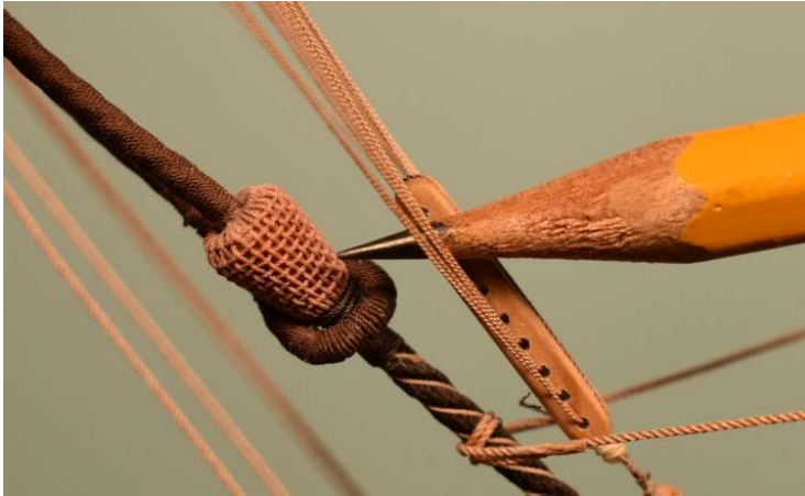
A "mouse" was created to prevent the fore stay collars from sliding up towards the masthead. Lloyd literally wove his miniature "mouse" using an over-under pattern.
