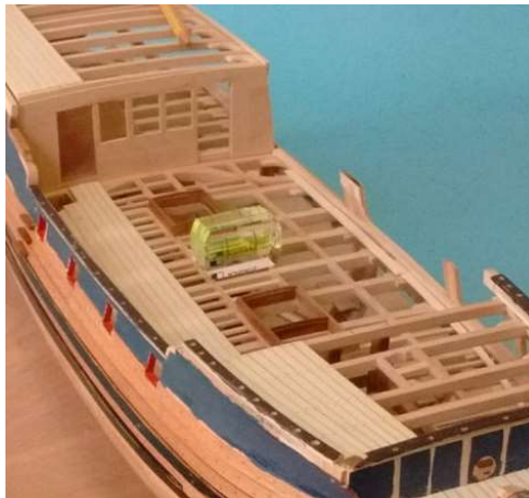
The deck planking is sprung in, not just glued down. Minimal deck planking is fitted, to allow unrestricted views below deck.
