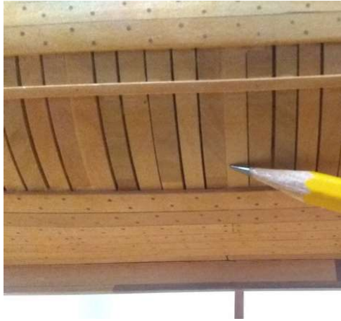
On the lower starboard hull the individual frames of the ship are visible. The center line of one of these bends can be seen at the point of the pencil.
