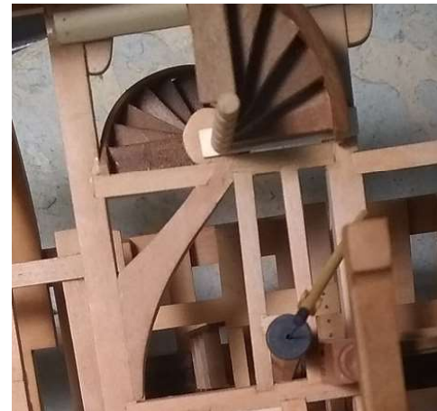
Twin staircases fit very nicely, though tightly, between the main deck beams and the spur beams.
