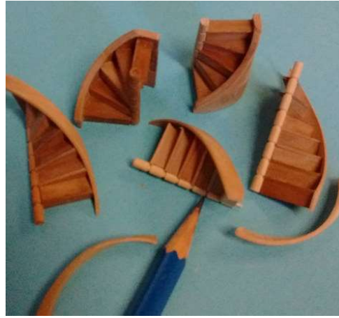
The 5 curving staircases were made in pieces then assembled to fit inside the model.
