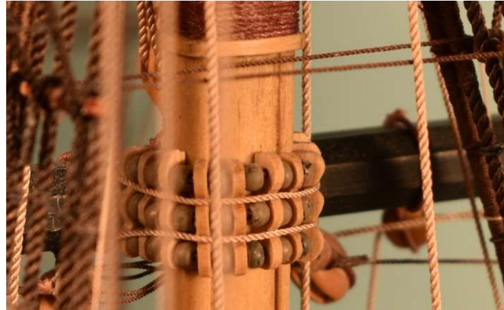
On the back of the lower mast the yard parrel holds the lower yard to the mast itself. The parrel is made up of round wooden trucks and spacers all held together by rope when they were braced around to the wind.
